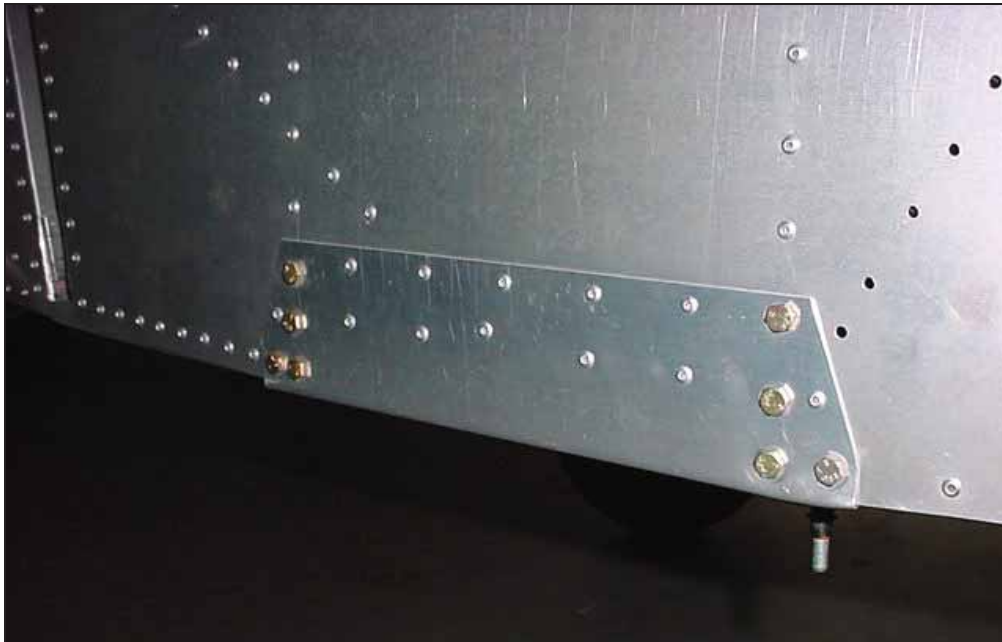
When converting tricycle to tail wheel, it is necessary to cover up the cutout with a plate.
