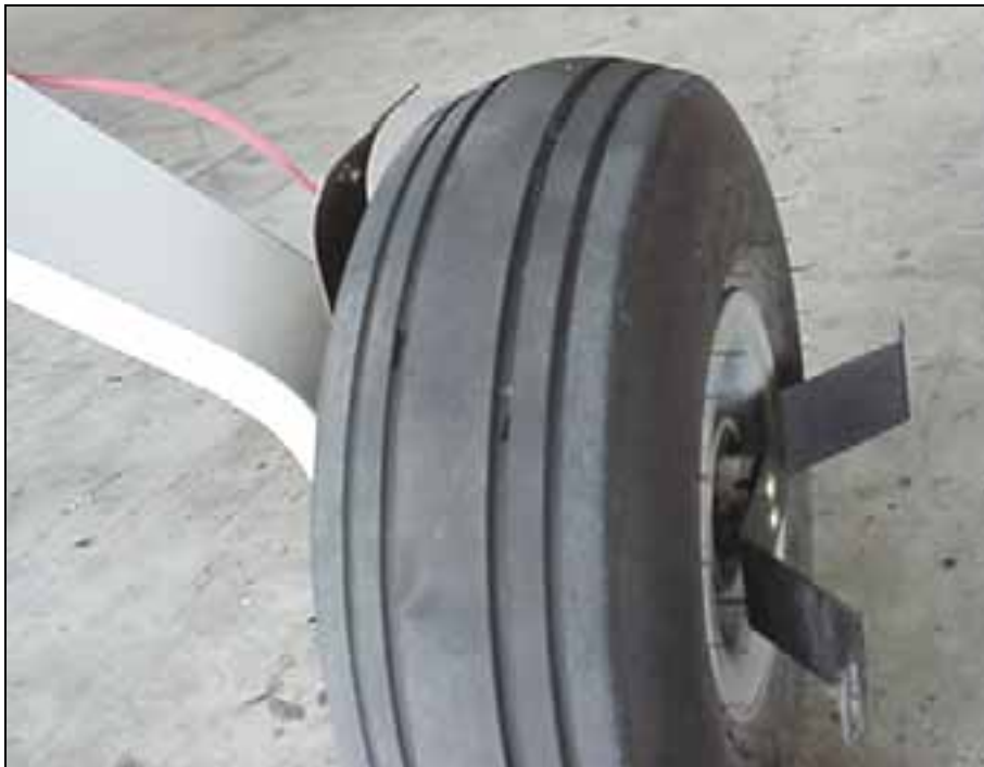
I/B and O/B wheel fairing attachment brackets
