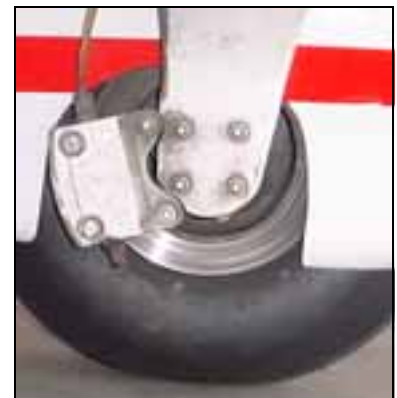
Inboard side of left wheel fairing, cutout for landing gear and brake calipers.
