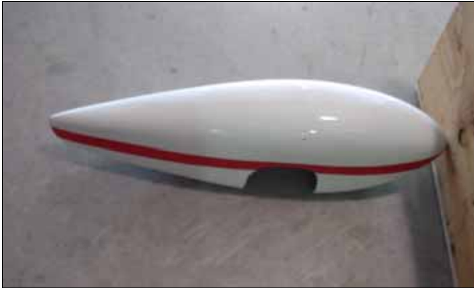
Position a wheel fairing with the nose against a wall.
