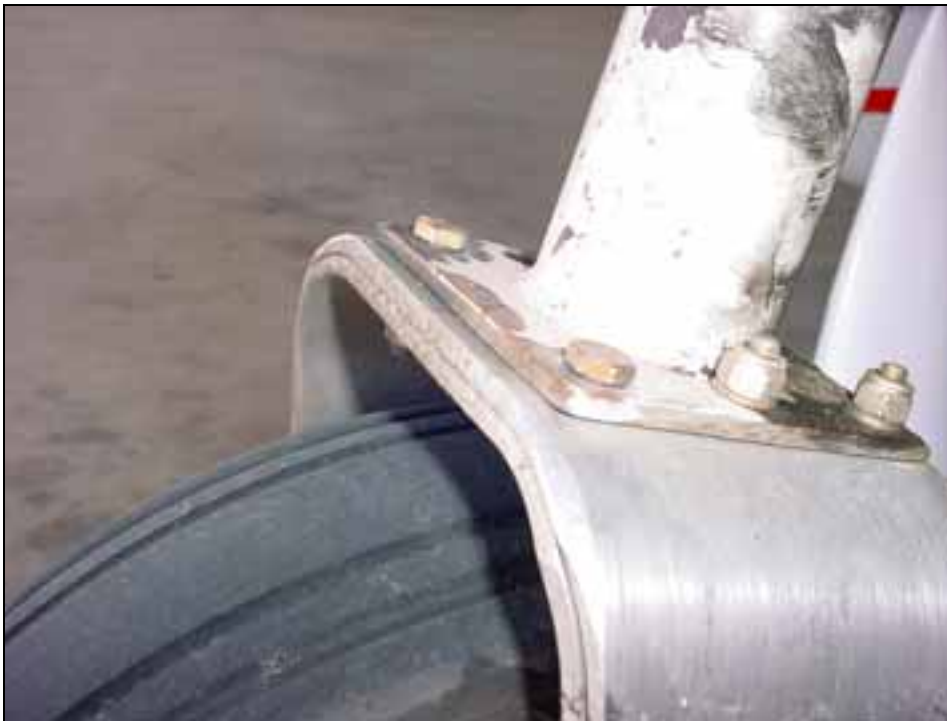
Detail of left side, filed radius along edge of fork doubler.
