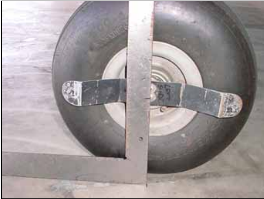
Use a square to mark the center of the main wheel axel on the floor.
