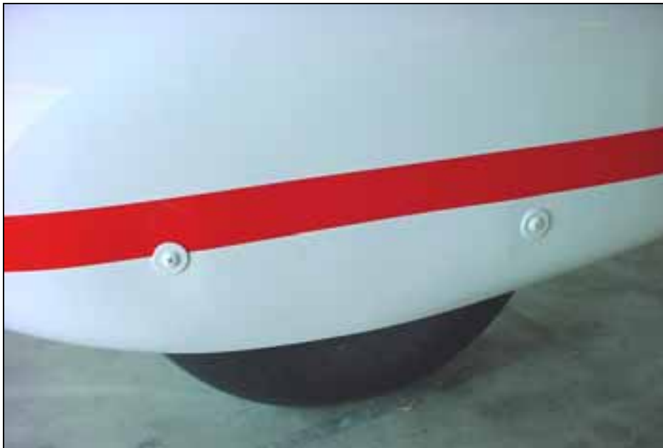
Two screws in each attachment bracket.
