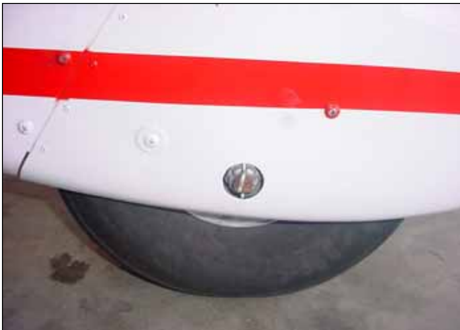
Drill 1" hole in the side of the wheel fairing for the nose wheel axel.
