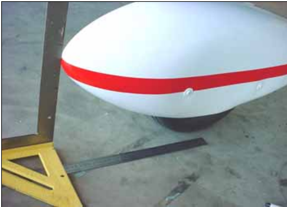
Check: distance from leading edge of fairing to center of main wheel axel
