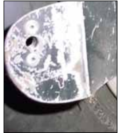
Hole in bracket with nut plate on the back side.
